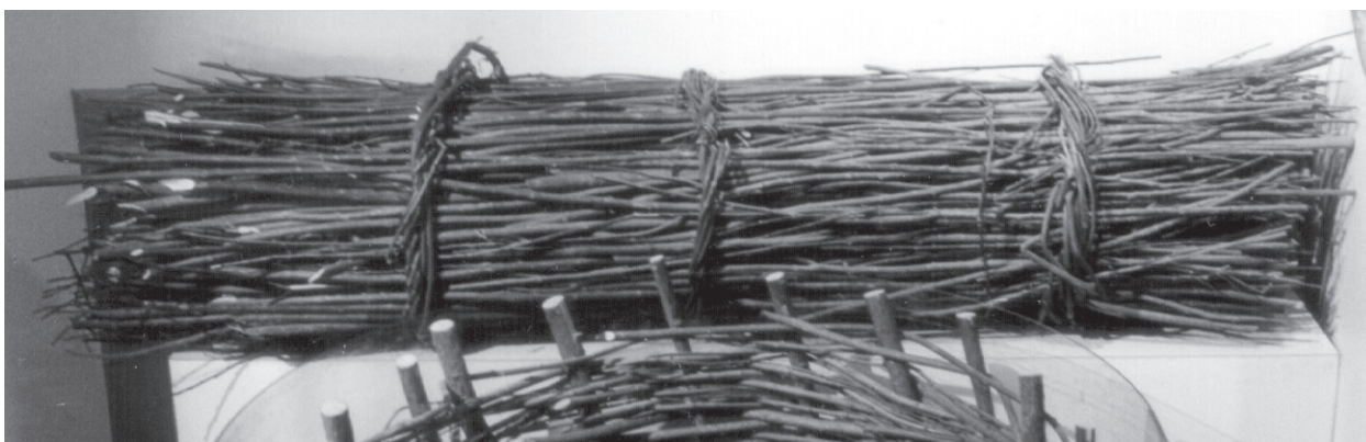
Figure 7.4. Modern example of a fascine.
