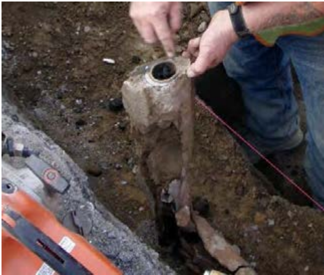
Photo 7.15: Segment of the pipe that broke at a narrow corroded spot. The sawed part shows the concrete lining the inside surface of the pipe as well as the thicker outer coating.
