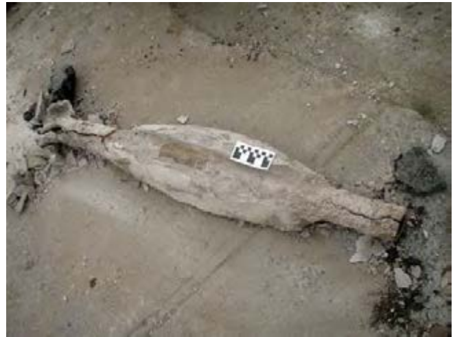
Photo 7.16: This meter-long pipe segment, removed from DRT 4, Unit 1 contained a pipe joint revealed after a strip of the thick part of the concrete was sawed away.
