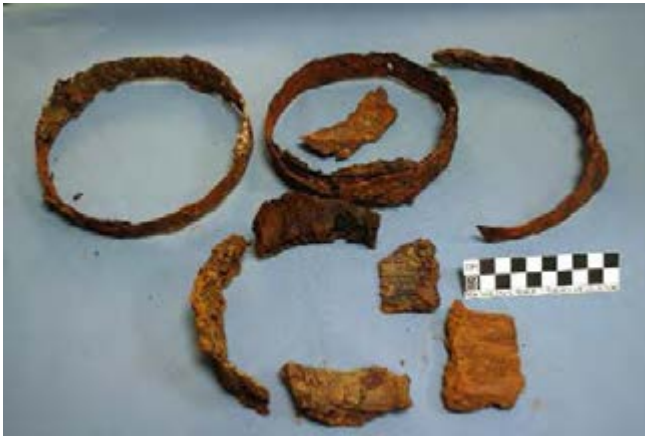
Photo 7.9: Iron straps found at the joints in the wooden water pipe in DRT 1 units.
